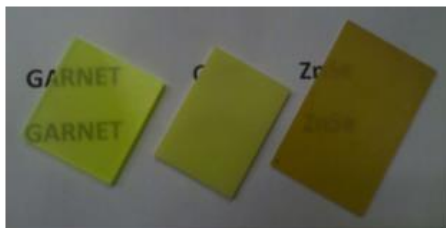
Fig. 10 Garnet-type (left), Gd_2O_2S:Pr,Ce (center), and ZnSe (right). Scintillator wafers (photo courtesy Philips Healthcare)
