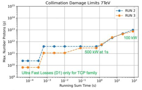
Maximum values of beam losses in the full collimation system.
