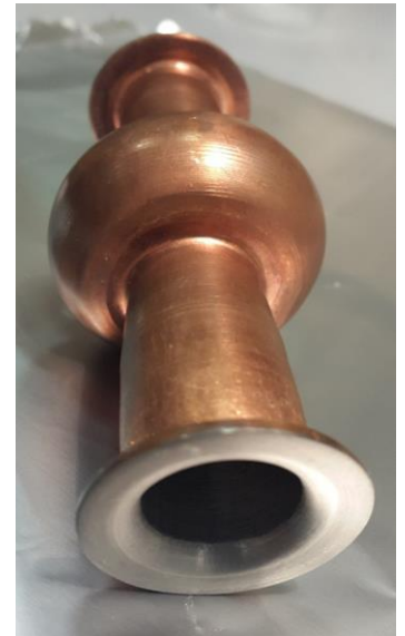
6 GHz Nb on Cu Cavity @LNL
