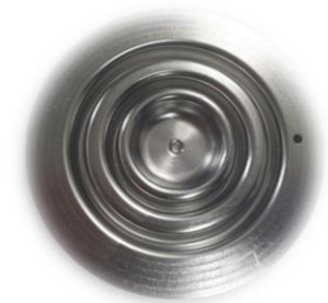
2 choke cavity at IJCLab for treatment
