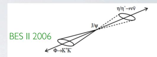
FIG. 1: Schematic of  $J/\psi \to \phi \eta$  or  $\phi \eta'$ . The  $\phi$ , which is reconstructed in  $K^+K^-$  final states, can be used to tag the invisible decay of the  $\eta$  and  $\eta'$ .
