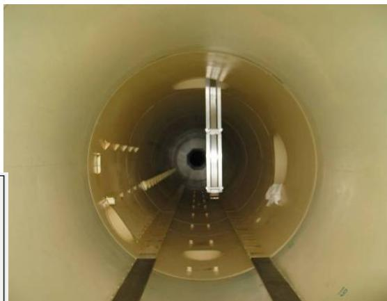
Small gap for diameter expansion under vacuum
