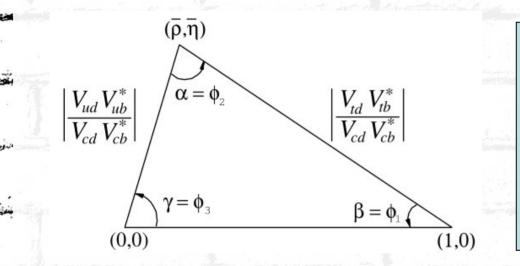
The angles can be written in terms of CKM matrix elements as:  $\alpha \equiv \arg[-V_{td}V_{tb}^*/V_{ud}V_{ub}^*]$   $\beta \equiv \arg[-V_{cd}V_{cb}^*/V_{td}V_{tb}^*]$   $\gamma \equiv \arg[-V_{ud}V_{ub}^*/V_{cd}V_{cb}^*]$
