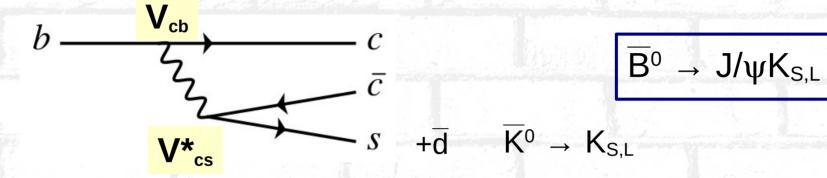
Here the CKM elements contributing are  $V_{cb}V_{cs}^*$  that have no phase. The CP conjugated case is also leading to (about) the same final state:
