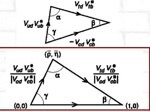
In terms of the Wolfenstein parameterization, the coordinates of this triangle are (0, 0), (1, 0) and  $(\overline{\rho}, \overline{\eta})$ : the two sides are  $(\overline{\rho} + i\overline{\eta})$  and  $(1 - \overline{\rho} - i\overline{\eta})$ . M.Bona – Flavour Physics – lecture 1
