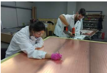
Drift Panel Cleaning
