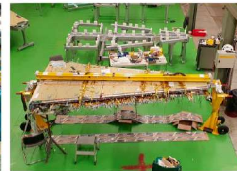
Integration chambers onto the spacer frame
