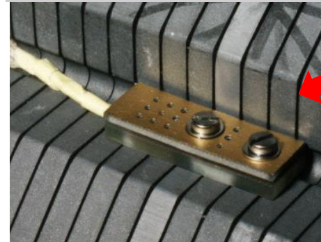
LHC cold mass thermometer. Mechanical protection for cable and fast flow
