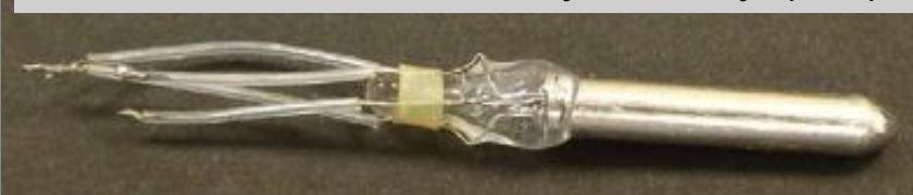
RIRT standard made by VNIIFTRI (RUS)
