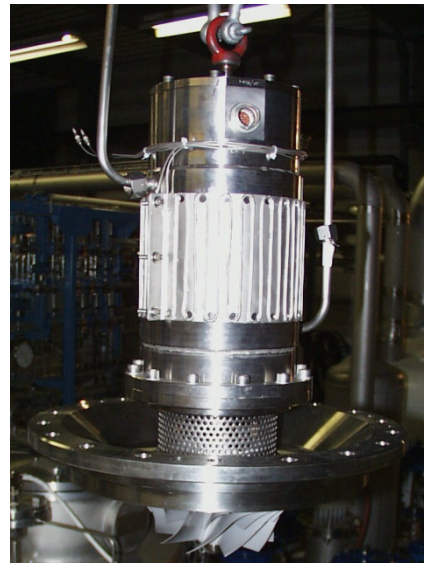
Fig. 18: Axial–centrifugal cold compressor cartridges for the LHC
