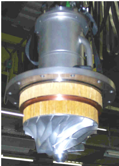
Fig. 18: Axial–centrifugal cold compressor cartridges for the LHC
