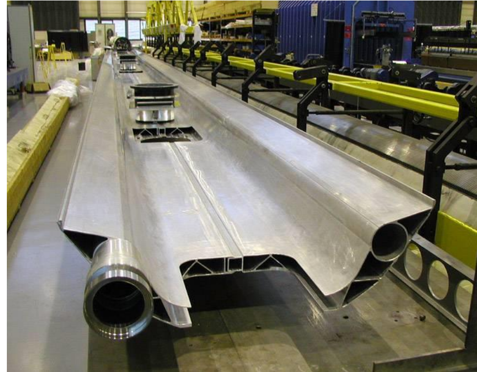
Aluminium alloy 6063 extrusions and 1100 top sheets
