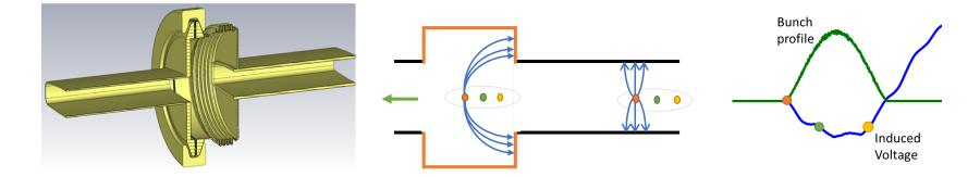
• A single particle passing through a cavity-like gap will induce a wakefield  $\mathcal{W}(\tau)$ . A bunch with a longitudinal charge density  $\lambda(\tau)$  (number of particles  $N_b$ ) will induce a voltage  $V_{\mathrm{ind}}(\tau)$ , as a convolution product of all the particles single wakes
