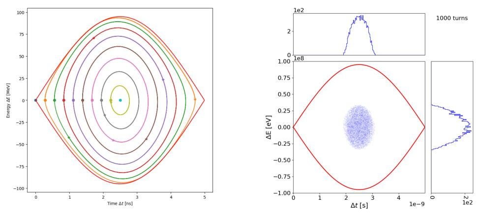
• Yesterday, we have experimented with longitudinal tracking by applying the two discretized equations of motion (energy gain and relative drift).
