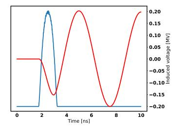
• The induced voltage can then be computed in time or frequency domain. In time domain, a numerical convolution is applied (e.g. *numpy.convolve*)
