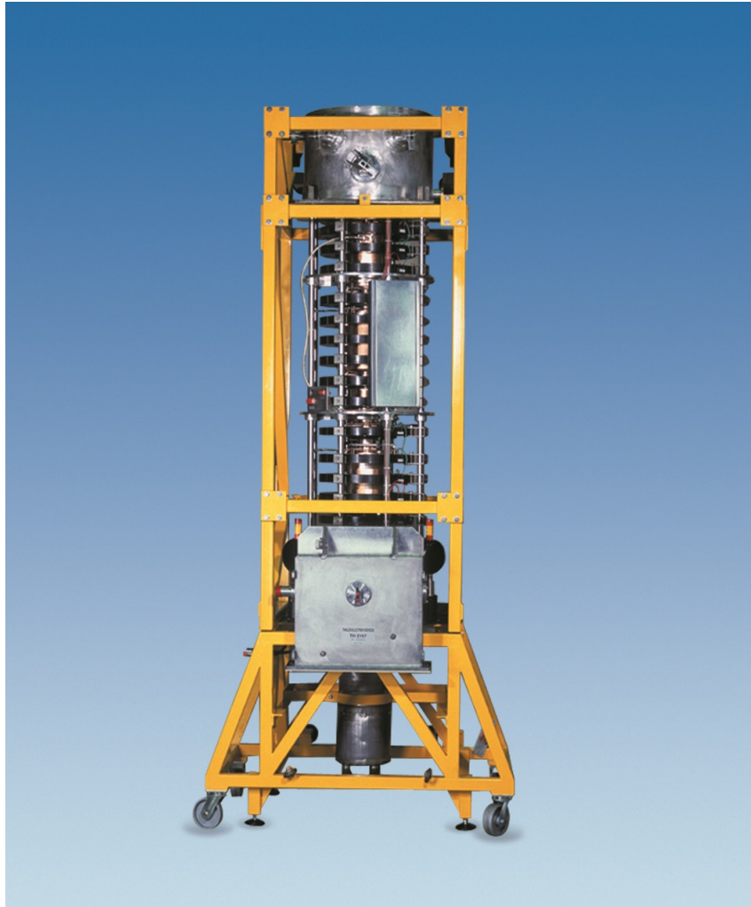
CERN LHC, TH 2167 klystron and in UX45 cavern 16 klystrons delivering 330 kW @ 400 MHz, into operation since 2008
