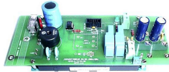
SOLEIL SYNCHROTRON elementary 600 W 300 Vdc / 30 Vdc converter board
