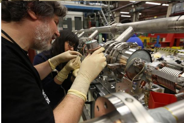
Tuner assembly, connection of linear actuator
