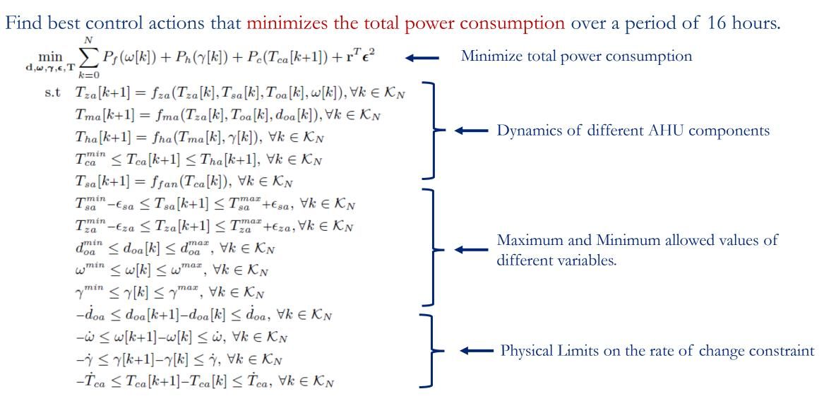
Output: Dampers Opening, Fan Speed, Heater Input, Cooled Air Temperature
