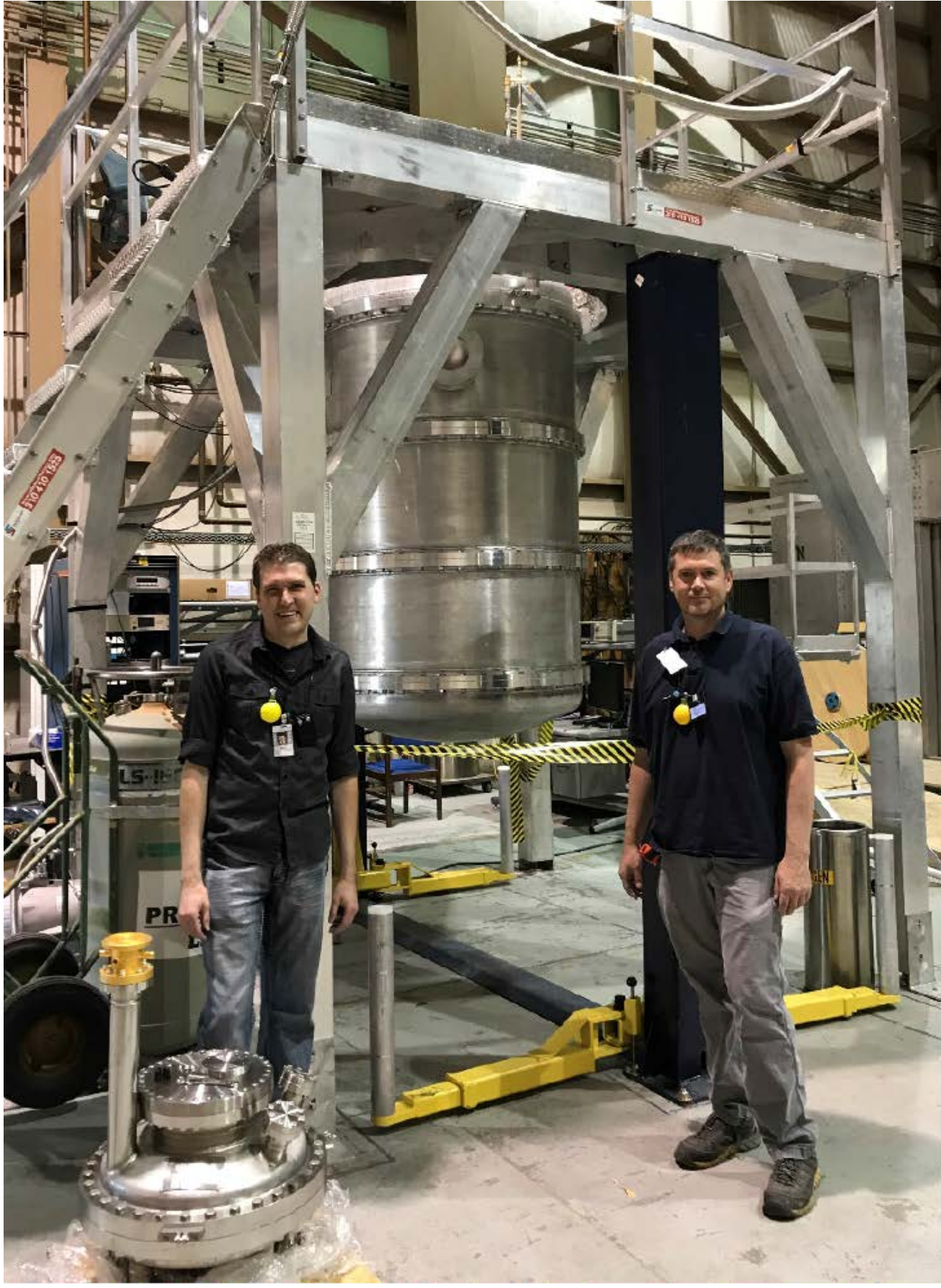
A half-scale electrode system is immersed in 40 liter LHe volume cooled to 0.4 K. HV performance test will be performed with 200 kV direct HV feed. The cryostat is currently being commissioned.
