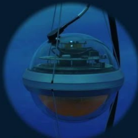
Digital Optical Module DOM 86 strings 5160 optical sensors
