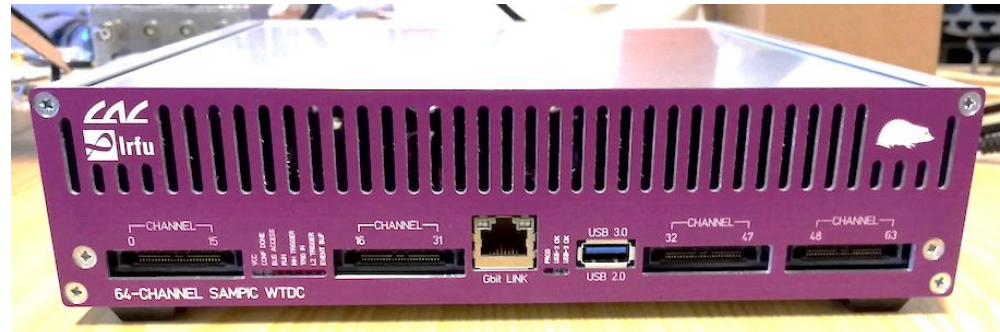
64-channel module with 16-channel input connectors (SAMTEC QRF8) (can be analog or differential digital) based on a 64-channel board
