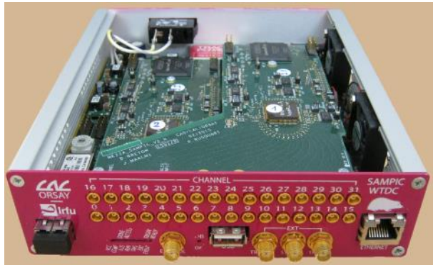
16 or 32-channel module (1 or 2 mezzanines)
