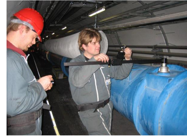
Manual device Accuracy 0.07mm
