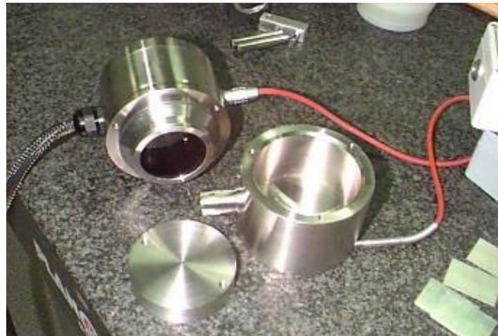
Hydrostatic Levelling Sensor (capacitive-based)
