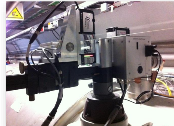
Automatic device Accuracy 0.1mm
