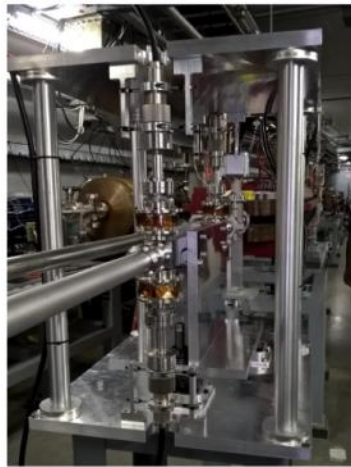
Figure 5: The kicker installed in the BTX beamline.
