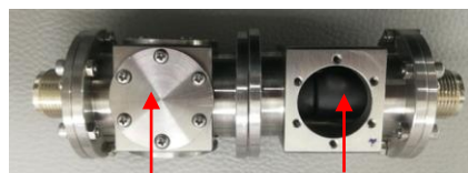
DSRD assembling (2×4=8pcs) Saturable inductor (2 DN200L ferrite cores)
