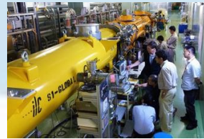
S1 Global: DESY, Fermilab, KEK 8-cavity string Test, 2010
