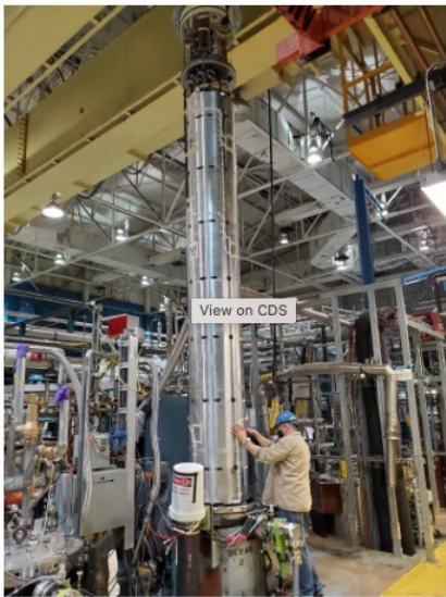
The MQXFA05 magnet enters the vertical cryostat at the Brookhaven National Laboratory for its endurance test (Image: BNL)
