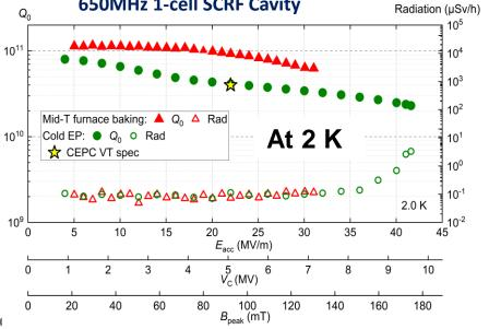
Q<sub>0</sub> = 6.0E10 @ 31 MV/m Q<sub>0</sub> = 2.1E10 @ 42 MV/m
