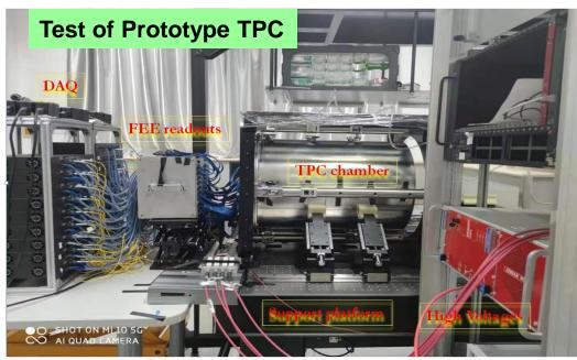
Challenge: Ion backflow (IBF) affects the resolution. It can be corrected by a laser calibration at low luminosity, but difficult at high luminosity Z-pole.
