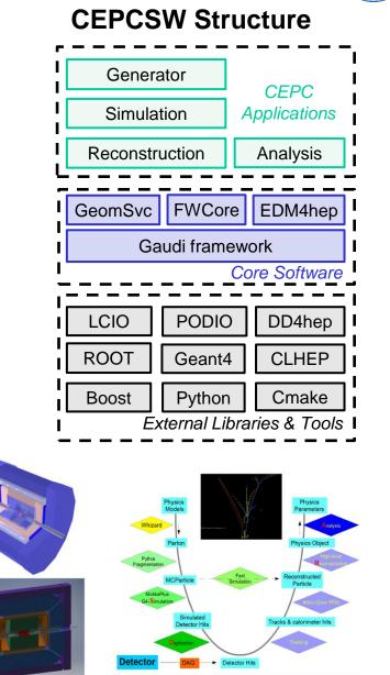
Full simulation reconstruction Chain functional, iterating/validation with hardware studies
