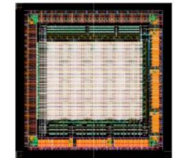
Develop **CEPCPix** for a CEPC tracker basing on **ATLASPix3 CN/IT/UK/DE** TSI 180 nm HV-CMOS process
