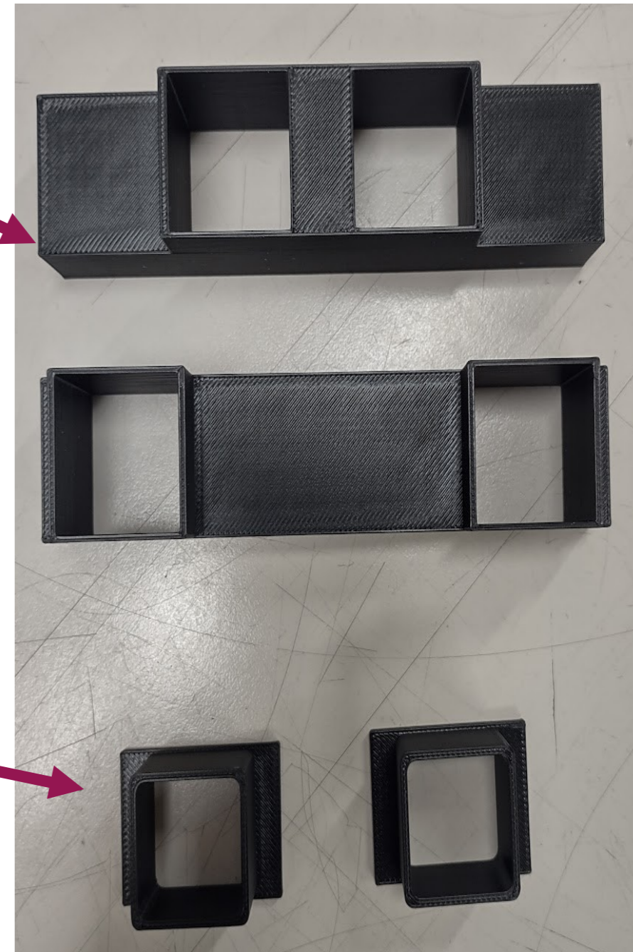
3D-printed fibre and PMT holders
