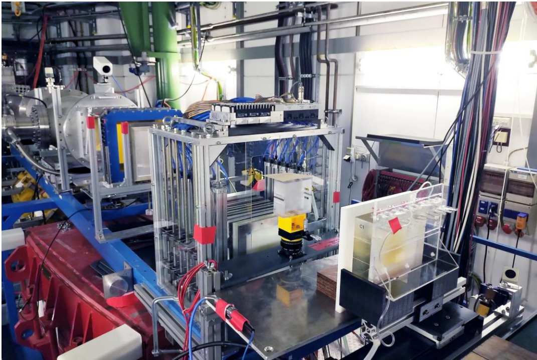
Setup: Preclinical irradiations (mice) for carbon FLASH experiments (2022)
