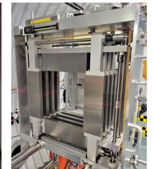
NSRL collimator system
