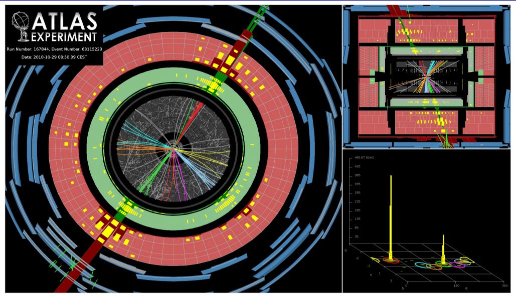
Highest- $p_{_{\rm T}}$  jet collected during 2010, which has  $p_{_{\rm T}}$  of 1.5 TeV. The two leading jets are central high- $p_{_{\rm T}}$  jets with an invariant mass of 2.8 TeV. They have  $(p_{_{\rm T}}, y)$  of (1.5 TeV, -0.58) and (1.0 TeV, 0.44), respectively. The missing transverse energy in the event is 310 GeV.
