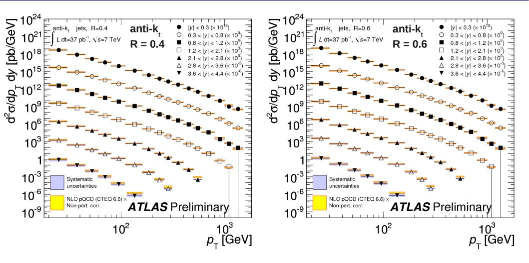
The inclusive jet cross section is measured from p<sub>+</sub> of 20 GeV to 1.5 TeV
