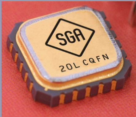
Hermetic QFN with ceramic package and sealed Kovar cover
