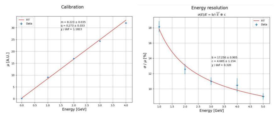
Figure 10: Linearity and energy resolution for electrons.
