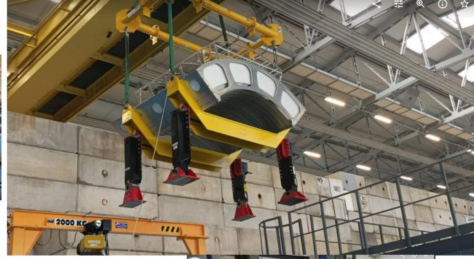
Movable platform "landing site" @ T9 test beam area.
