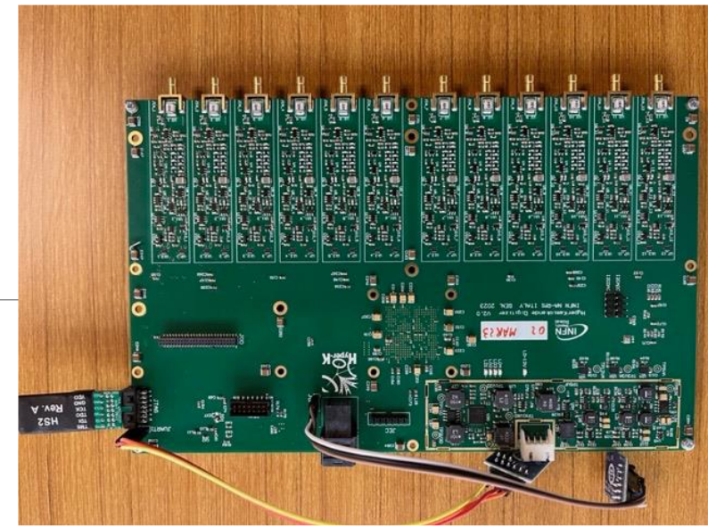
ID 12 channel-front end board
