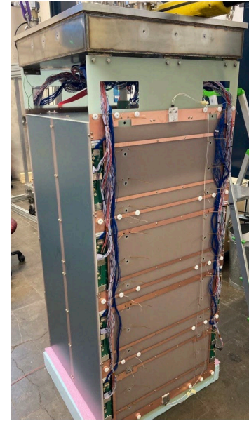
DUNE Near Detector Prototype LArTPC
