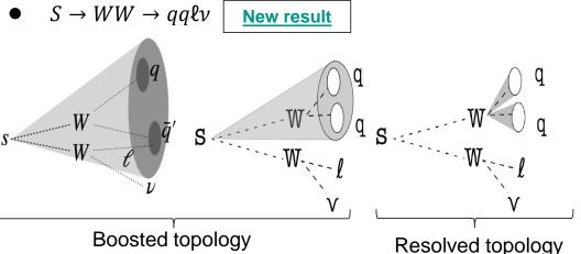
Special technique to reconstruct boosted hadronically decaying *W*
