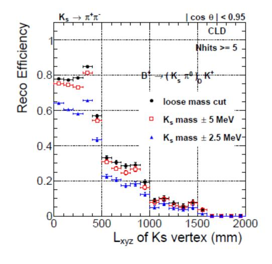
Large tracking volume with many measurement points is very important for Ks reconstruction
