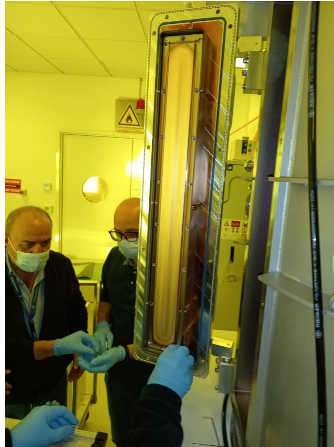
70cm copper target installation
