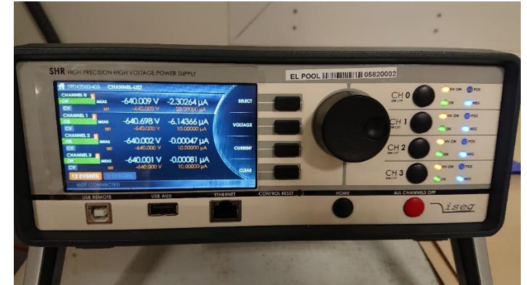
HV Power supply 10 to 20uA limitation
