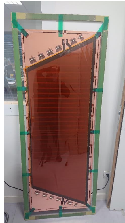
CLAS12 uRwell 2D PEP with 3 CS layers Active area: 150cm x 50cm
