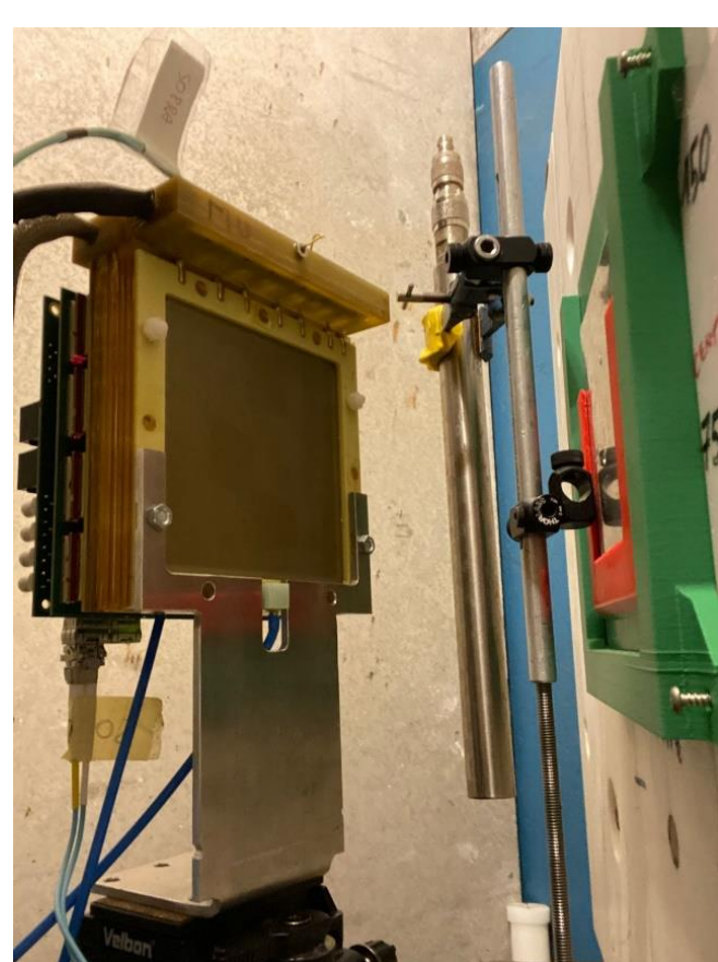
Figure 2. 3-MBGEM detector at TRIGA Mark II reactor in Pavia.
