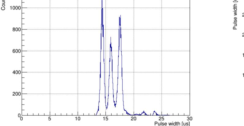
2D plot of pulse width versus pulse area and their axis projection spectra for alpha particles from <sup>233</sup>U (4.8 MeV), <sup>239</sup>Pu (5.2 MeV) and <sup>238</sup>Pu (5.5 MeV) source, measured in low-pressure TPC in isobutane at 50 torr and THGEM gain of 320
