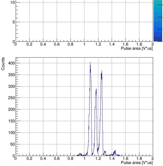
One can see that the use of GEM instead of THGEM substantially improve the energy resolution at a nominal pressure (50 torr).
