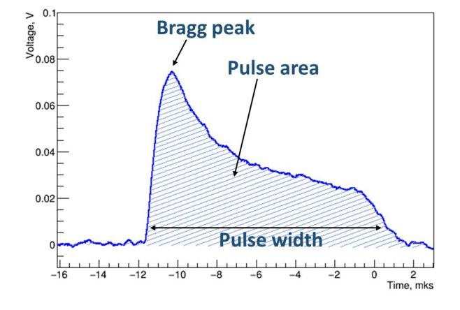
Signal waveform from alpha particle: pulse width ~ track range pulse area ~ energy
