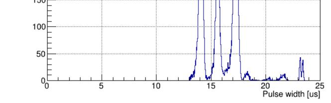
2D plot of pulse width versus pulse and their axis projection area spectra for alpha particles from <sup>233</sup>U (4.8 MeV), <sup>239</sup>Pu (5.2 MeV) and <sup>238</sup>Pu (5.5 MeV) source, measured in low-pressure TPC in isobutane at 50 torr and GEM gain of 230
