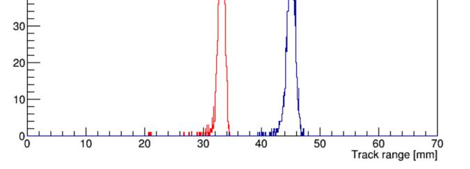
Track ranges distribution of 4 MeV <sup>10</sup>Be and <sup>10</sup>B for 200 nm silicon nitride window and 50 torr isobutane, obtained using SRIM simulation
