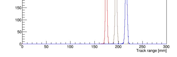
Track ranges distribution of alpha particles with different energies for 200 nm silicon nitride window and 50 torr obtained isobutane, using SRIM simulation
