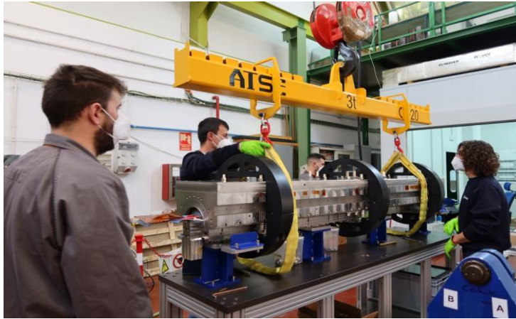
Assembly of inner coil impregnation mould
