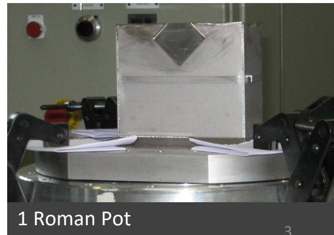
Si edgeless detector of the DO - TOTEM experiment
