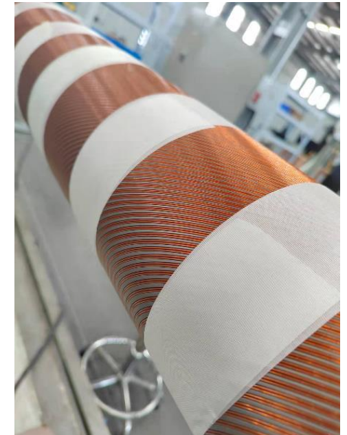
Canted Cosine Theta Corrector production from IHEP/Bama in China
