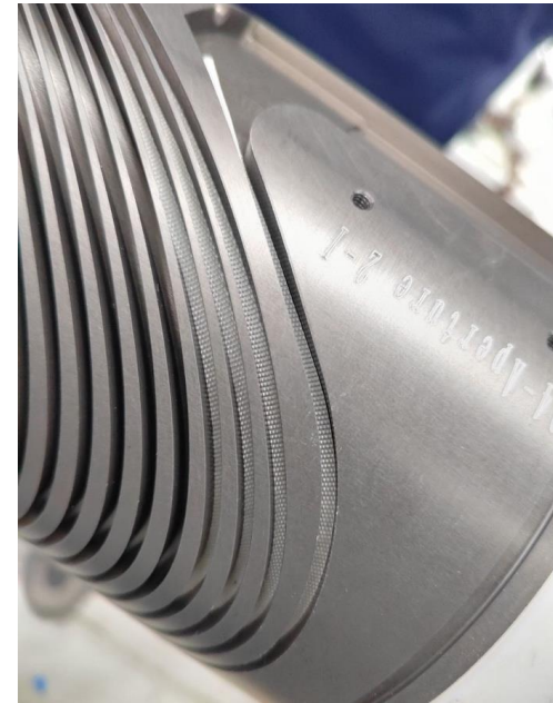
Canted Cosine Theta Corrector production from IHEP/Bama in China
