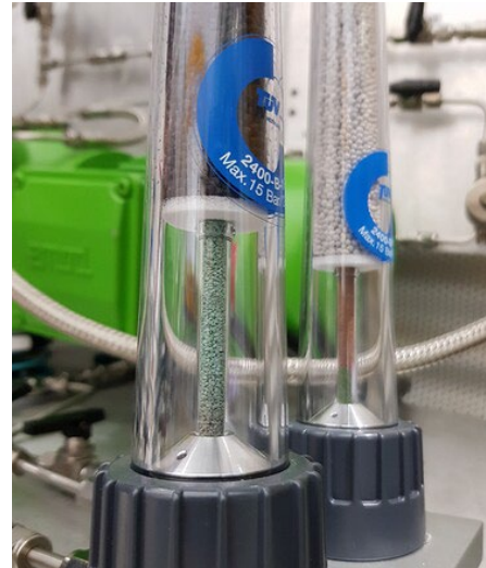
Testing radon emanation of commercial and home-made moisture filters
