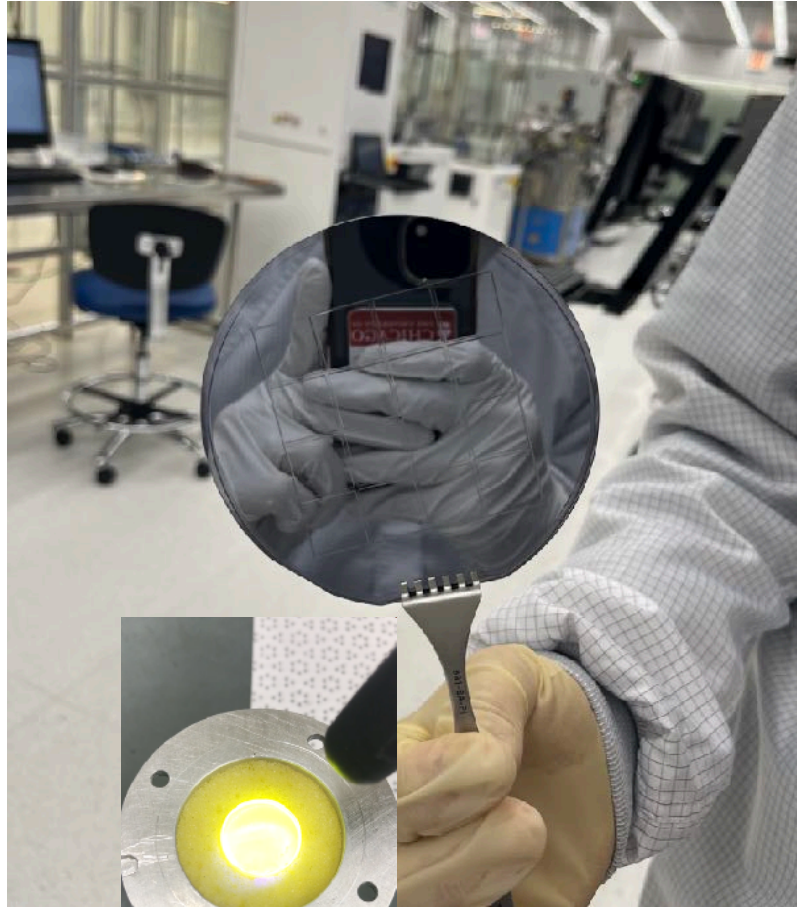
NOL-9 waveshifter exit plate illuminated by 360 nm UV LED. (see arXiv:1911.00762)
