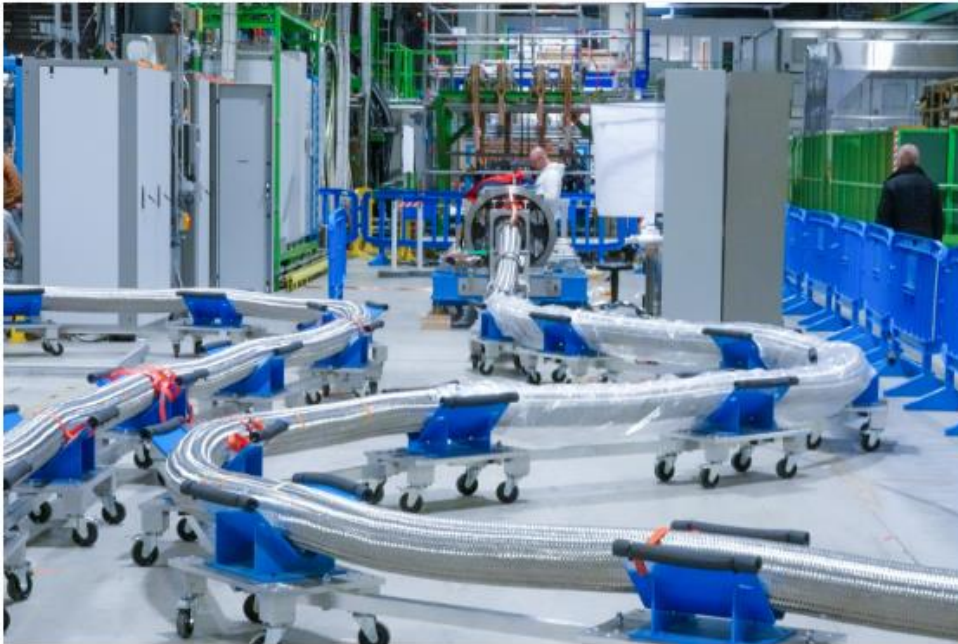
A novel, flexible cryostat, colloquially known as the "python", composed of 19 high-temperature magnesium diboride superconducting cables that can carry 120 kA. (Image: CERN)
