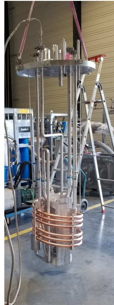
Caption : Photography of the 3 heat exchangers
