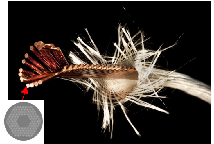
Nb 3 Sn Rutherford cable. Source: [CERN]
