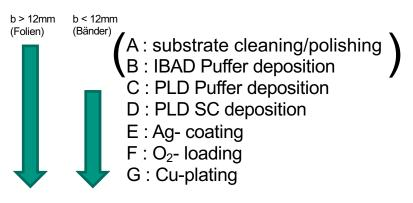
+ characterization (structural, electrical, mechanical)
