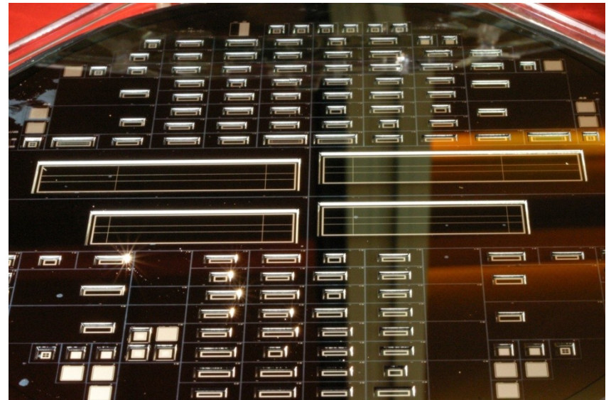
DEPFET active pixel sensors for Belle II Wafer before cutting (50 μm thick)
