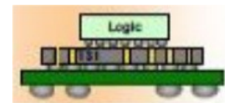
Silicon Interposer to high Integrated MCM
