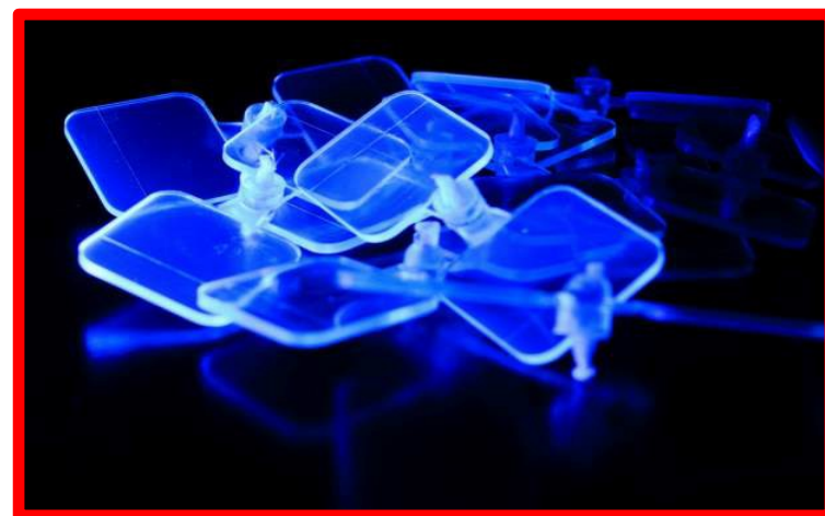
Production of PET and PEN scintillators for FCC detectors Collaboration with Institute for Polymers and Composites Uni. Minho
