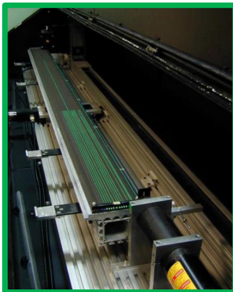
WLS/scintillating Optical fibre characterisation with LED
