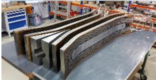
2018: FRESCA2 14.6 T at 1.9 K 100 mm bore
