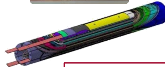
CEA cos-theta magnet, insulated and impregnated
