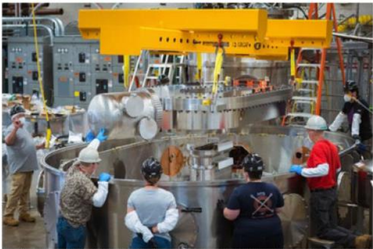
A team of engineers and scientists from CFS and MIT's PSFC lower the superconducting magnet into the test stand in which the magnet was cooled and powered to produce a magnetic field of 20 tesla. COMMONWEALTH FUSION SYSTEMS
