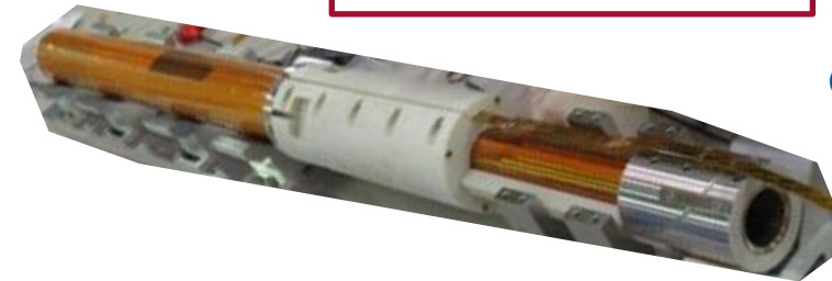
CEA cos-theta magnet, insulated and impregnated
