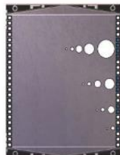
SDD: 2 \times 112 anodes, pitch = 970\mu\text{m}
