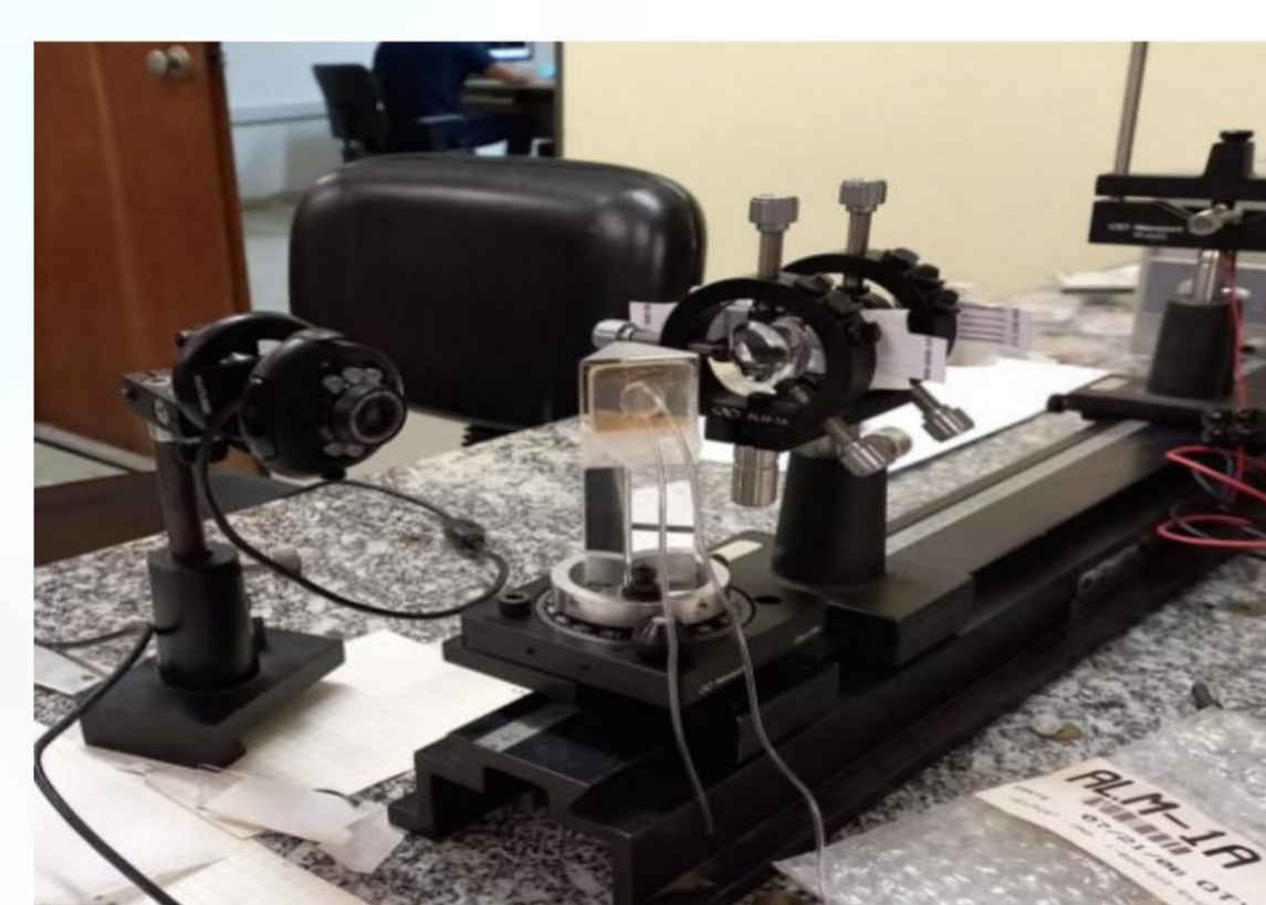
Figure 7: Prototype based on a system composed of lenses, laser and prism
