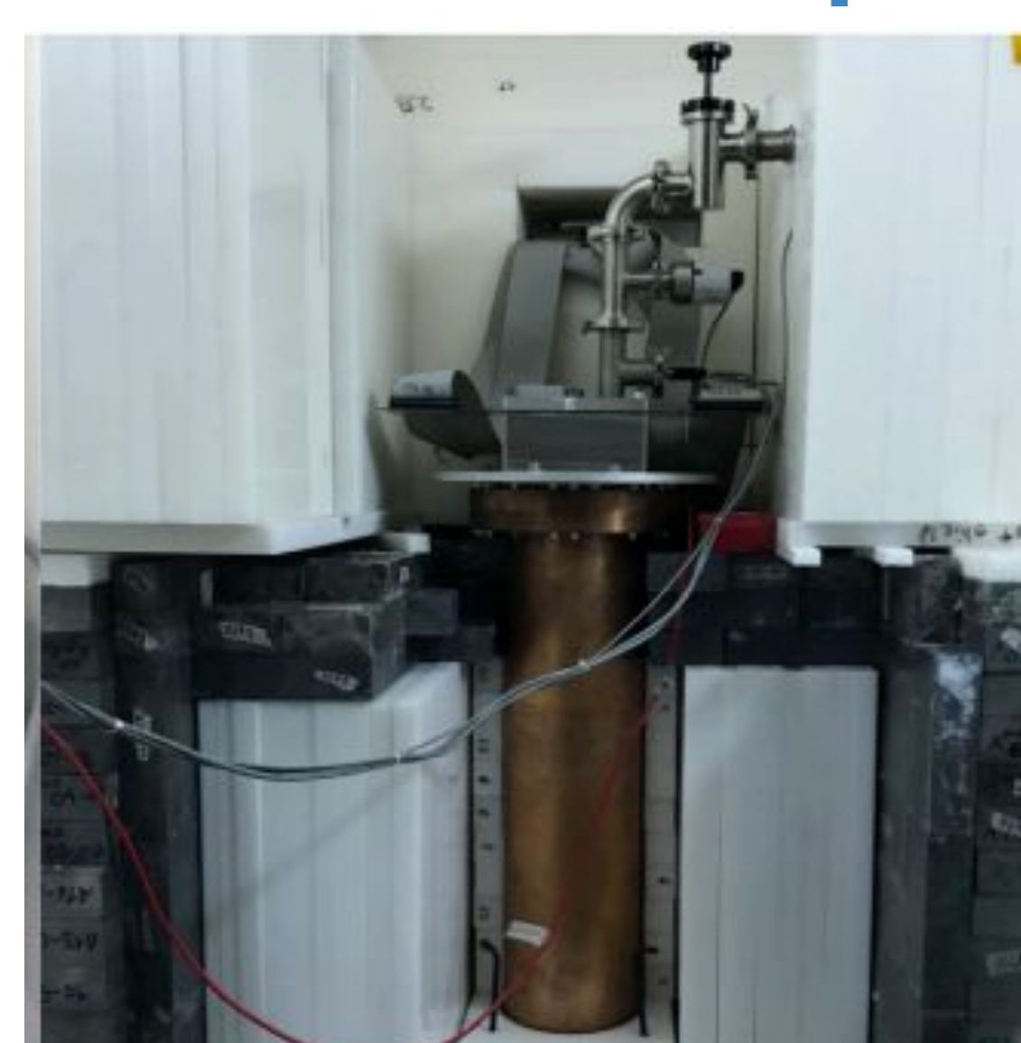
Fig 5. A view of the CONNIE detector and its shielding.
